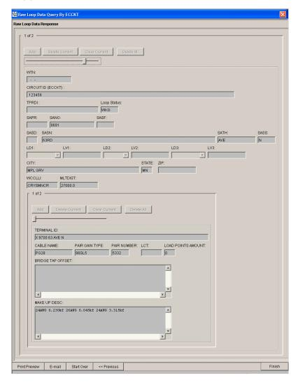
The bottom of the **Raw Loop Data Response** window shows the physical characteristics of the loop.
